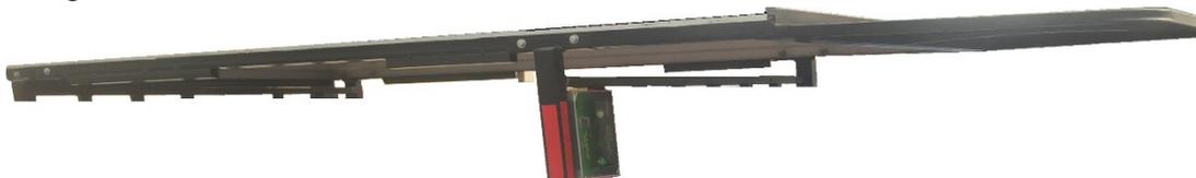
**The dimension of Solar PV module is within outer limits defined by I-CAT for E rickshaw roof (W:990mm).**
